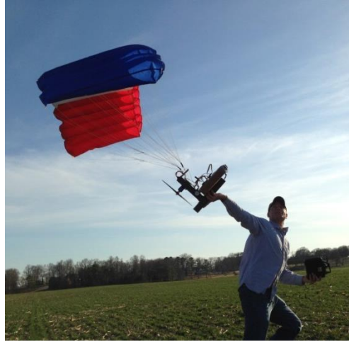
Fig. 7. Photo of Experimental Parafoil-Payload System with Embedded GPU (located in brown box on payload).
