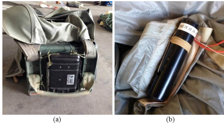
Figure 18: (a) Payload relay box mounted on MC-4/5 AGU, and (b) in-canopy actuator mounted within MC-4/5 canopy prior to test flight.
