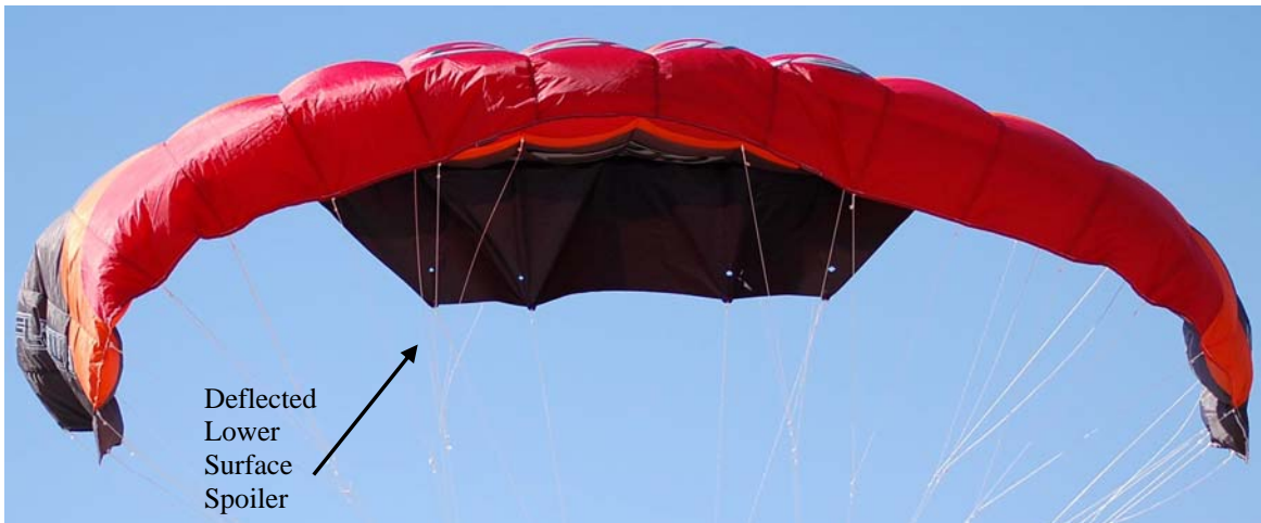
Figure 4. Lower Surface Flap Spoiler on Test Flight Canopy
