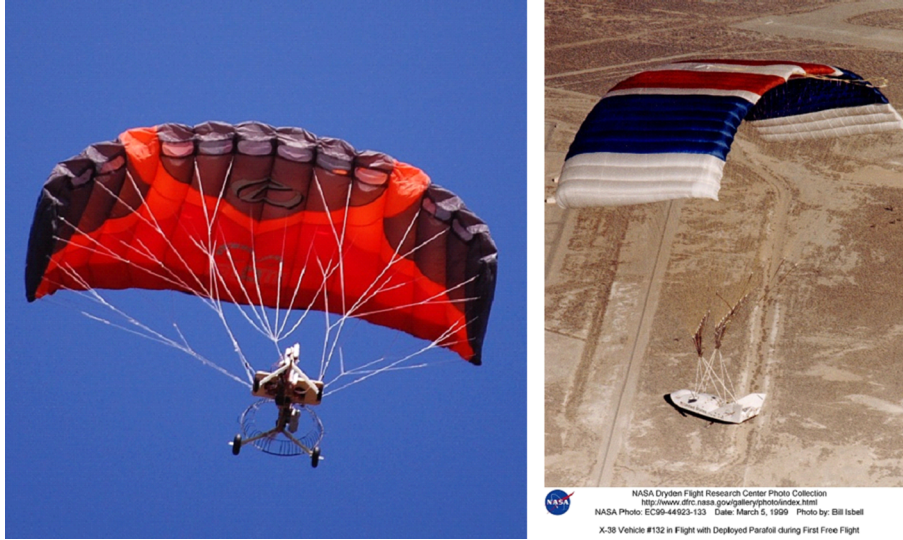
Fig. 6 Example parafoil systems: GT Imp (left) and X-38 (right).
