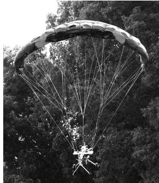
Fig. 15 LE collapse under large forward spoiler deflection.
