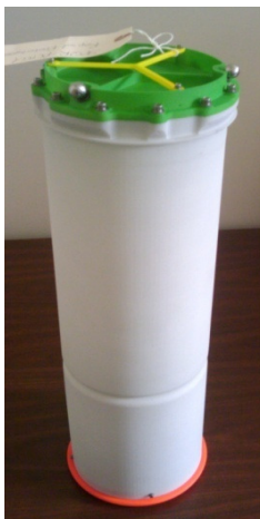
Fig. 11: Phase Change Thermal Control Unit integrated module (model)
