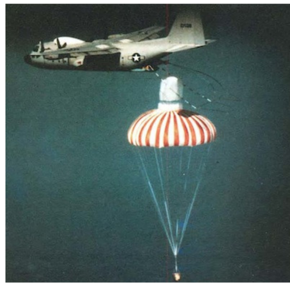
Figure 4. KeyHole satellite film mid-air recovery. (Credit: National Reconnaissance Office)
