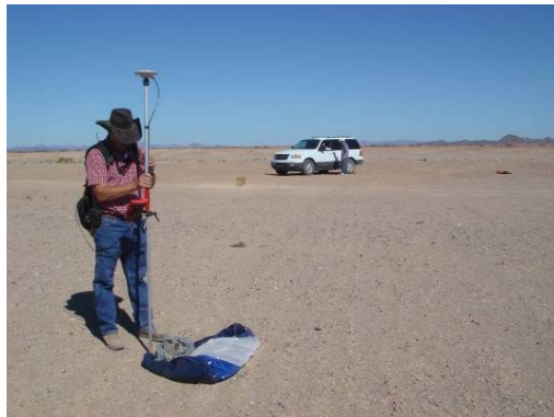
Fig. 17 Geodetic survey of the touchdown point.
