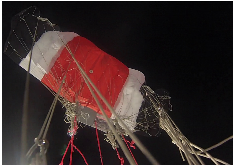
Figure 18: Large canopy fully inflated at high altitude with control lines tangled on payload.
