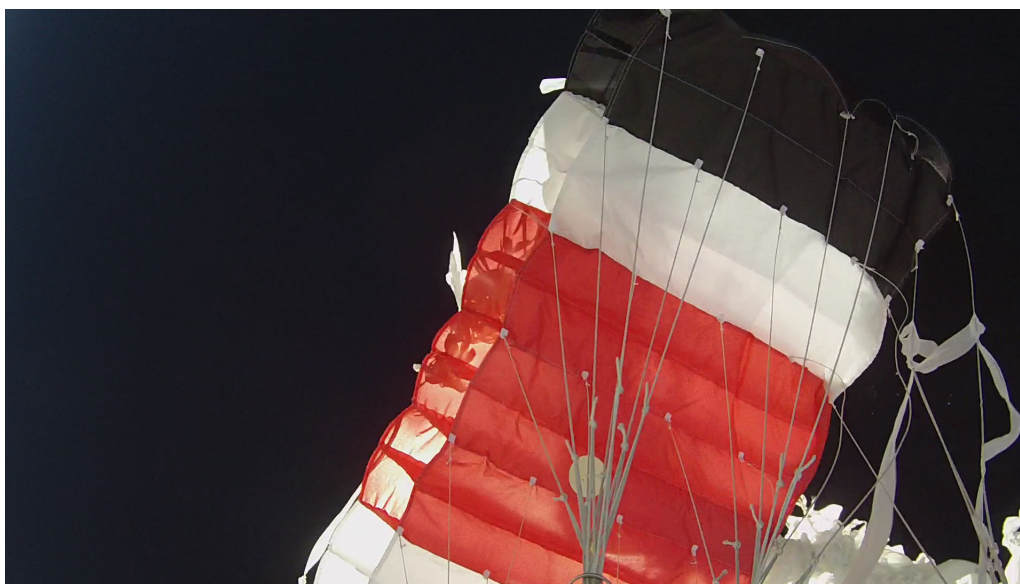
Figure 12: Upwards facing camera showing full canopy inflation after balloon burst (altitude \approx 26.6 \text{ km} ).
