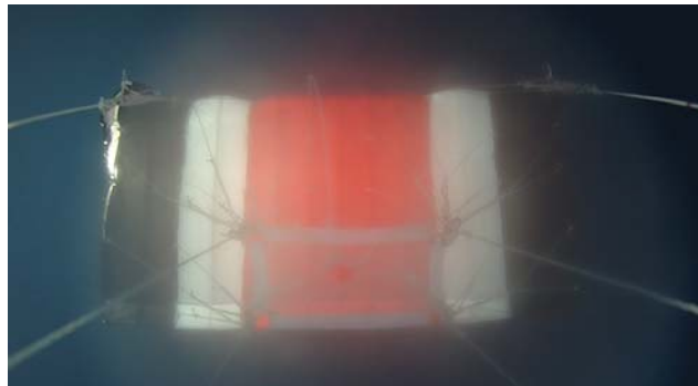
Fig. 30. View from the up-looking camera after successful parafoil inflation at 50,000ft altitude ASL.
