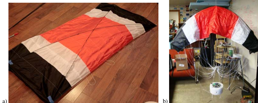
Fig. 8. Parafoil stiffening structure test-fitted to parafoil (a), suspended parafoil remains open, yet highly flexible under its own support (b).
