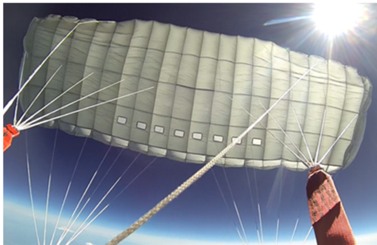
Figure 24. Canopy Surge (Predecessor to Overspeed Condition)
