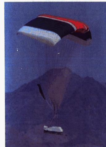
Figure 10. Doghouse test article under a 7,350 sq ft parafoil.
